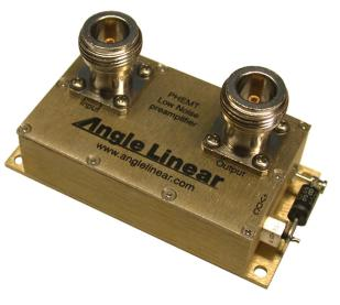
Construction is rugged: an irridited aluminum enclosure with stainless steel hardware throughout. Twenty screws attach the covers and give maximum shielding for the most hostile RF environments. TriMetal plated connectors have ptfe (Teflon) dielectric with gold pins and are available in type N, TNC and SMA (ss). Dimensions: 1.5"x 2.5"x 0.7". Mounting and connector positions give maximum versatility for high density rack panel mounting.
